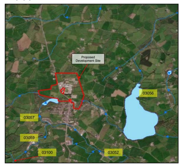
Gauging Stations 03057 (Emyvale Weir) and 03100 (Derrynashallog) are located on the Mountain Water River and are registered as active staff gauges and record either water level and/or flow data.
